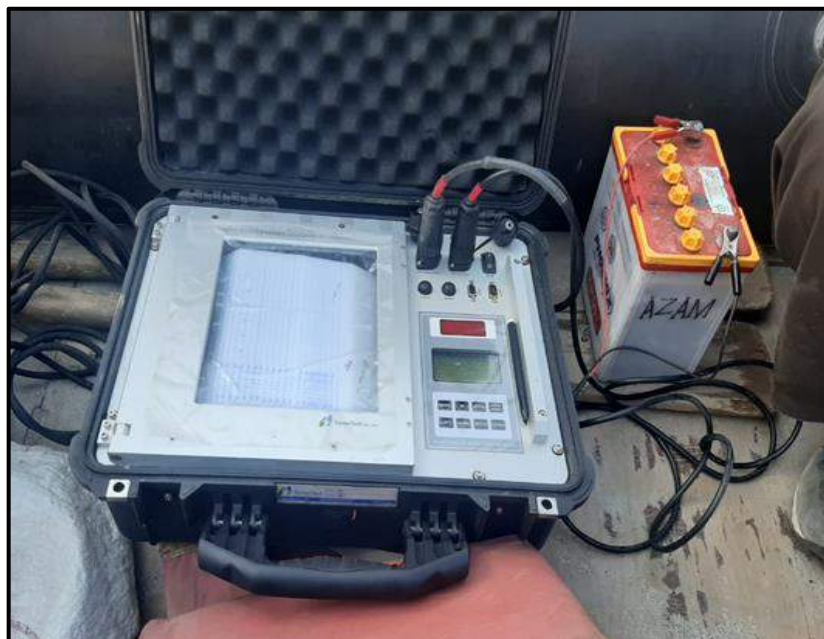
Figure 3-10 Equipment showing continuous Trace of Bed Profile
